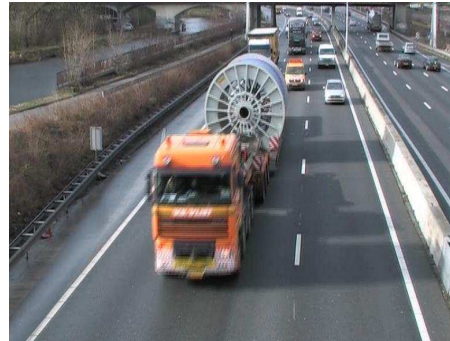
Figure 2: 400kV XLPE drums transported by truck
